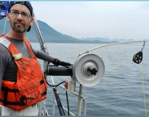
Above: NOAA Teacher at Sea Rob Ulmer uses a winch to cast a CTD (conductivity, temperature, & depth sensor) from NOAA ship Rainier .
