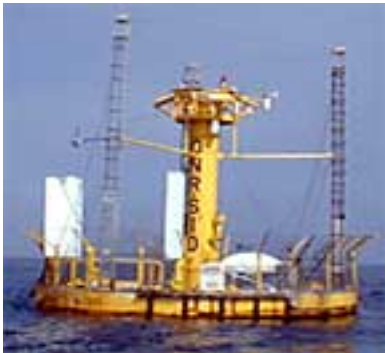
First test of a radar wind profiler on a 10-m discus buoy
