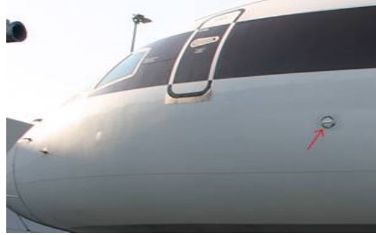
Mounted flush on the side of 25 UPS (B-757) aircraft, the air sampler produces little in-flight drag. (Photo courtesy UPS)
